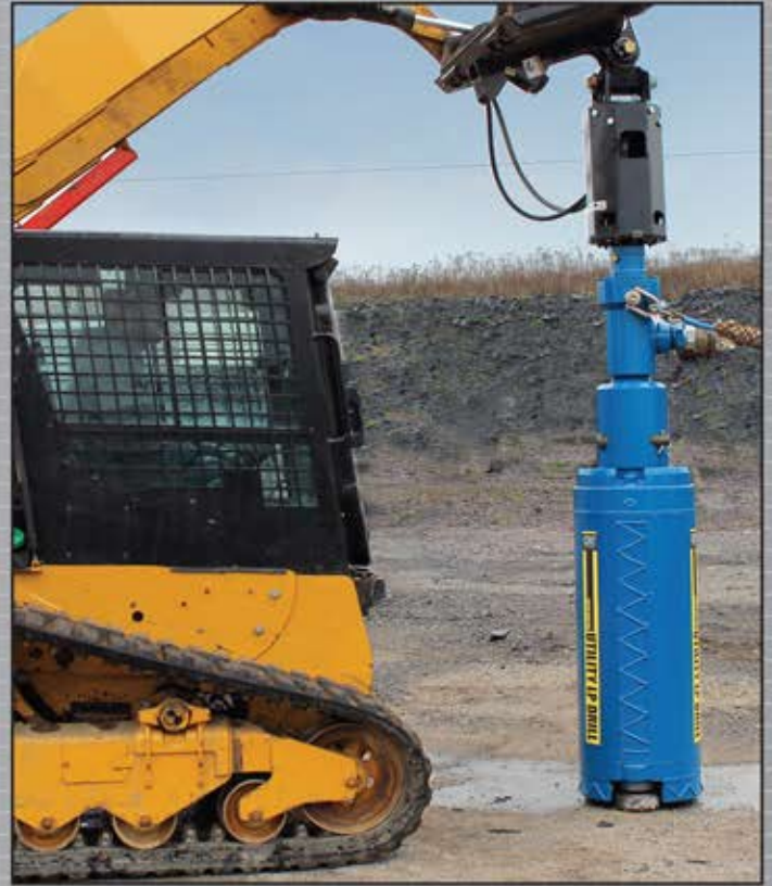
The LP drill mounted on a skid steer.
