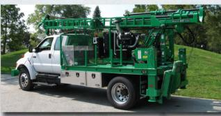
The D-50 is our premiere, all-purpose drill rig for the environmental and geotechnical drilling industry. With up to 9,000 ft lbs of spindle torque, it can power through most any job! Whether it is the D-50's ability to be mounted on a variety of carriers, or its superior drilling capability with augers, soil sampling, coring or probing, you can be sure you have a versatile drill that has the ability to get you where you need to go and the power to get the job done!
